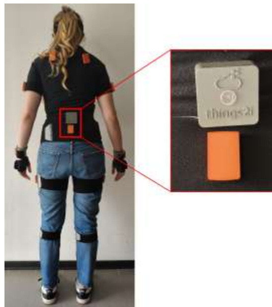
Figure 4. Placement of the move2i ® and XSens MVN Awinda system. The MVN Awinda sensors are attached with velcro straps on specific body locations, and the move2i ® device is placed on the lower back.
